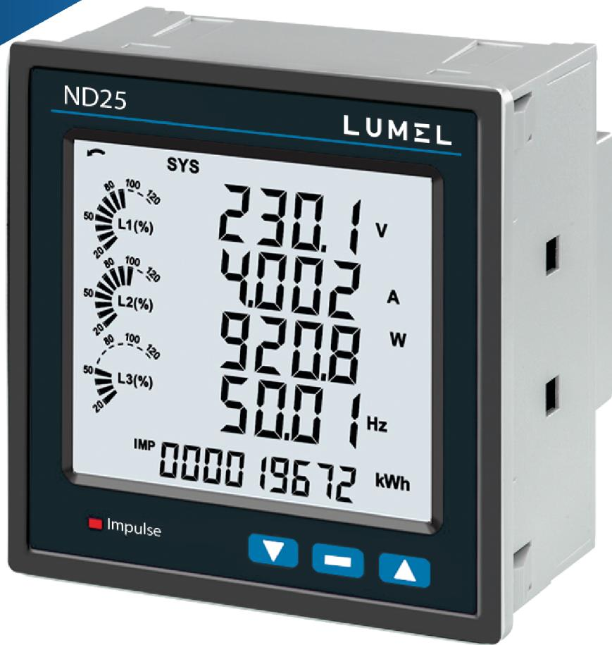
**ND25** measures important electrical parameters in 3 phase 4 wire, 3 phase 3 wire and 1 phase 2 wire Network. It displays many parameters at a glance. It measures electrical parameters like Active / Reactive / Apparent energy , power and all basic parameter. The instrument has two optional outputs. It can be configured as pulse output for energy measurement , limit output , timer function and RTC relay.
