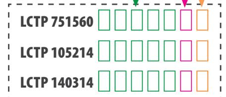
Ordering example: Order code LCTP 7515600150A55 means the transformer LCTP 75/15(60) 150/5A; Class 0.5; power 1.5VA
