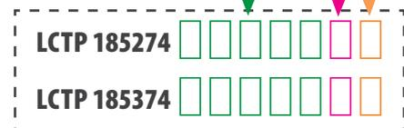
Ordering example: Order code LCTP 1852740150A51 means the transformer LCTP 185/27(45) 150/5A; Class 1; power 1.5VA
